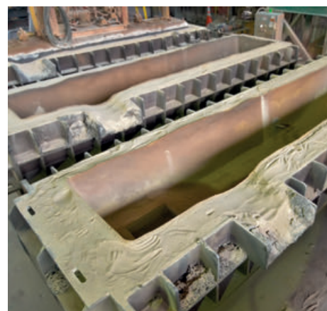
Tundishes with TUNDEX vibratable material
